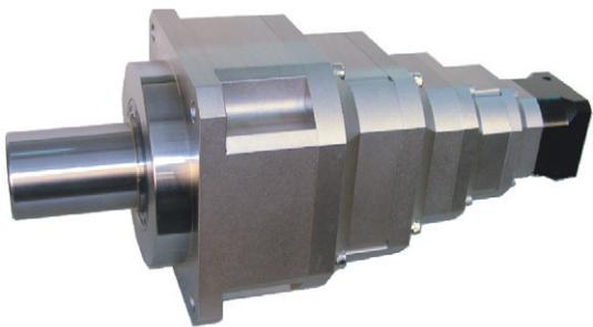
RATED OUTPUT TORQUE : Under the rated loading and long time running conditions, the allowable output torque for a gear reducer. The maximum output is the triple of this value.
